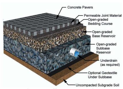
Figure 1 - Permeable Pavement Cross Section
